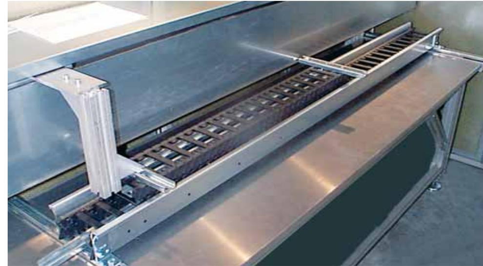
Noise test in the igus® laboratory 40db(A) E6.29.100.100.0 series for long travel paths, v = 2 m/s
