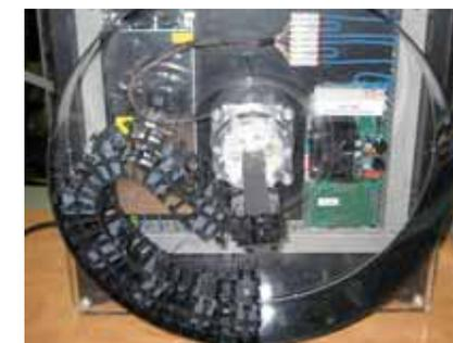
Standardised modules for rotational movements with the T3 system. Various sizes available in a short time
