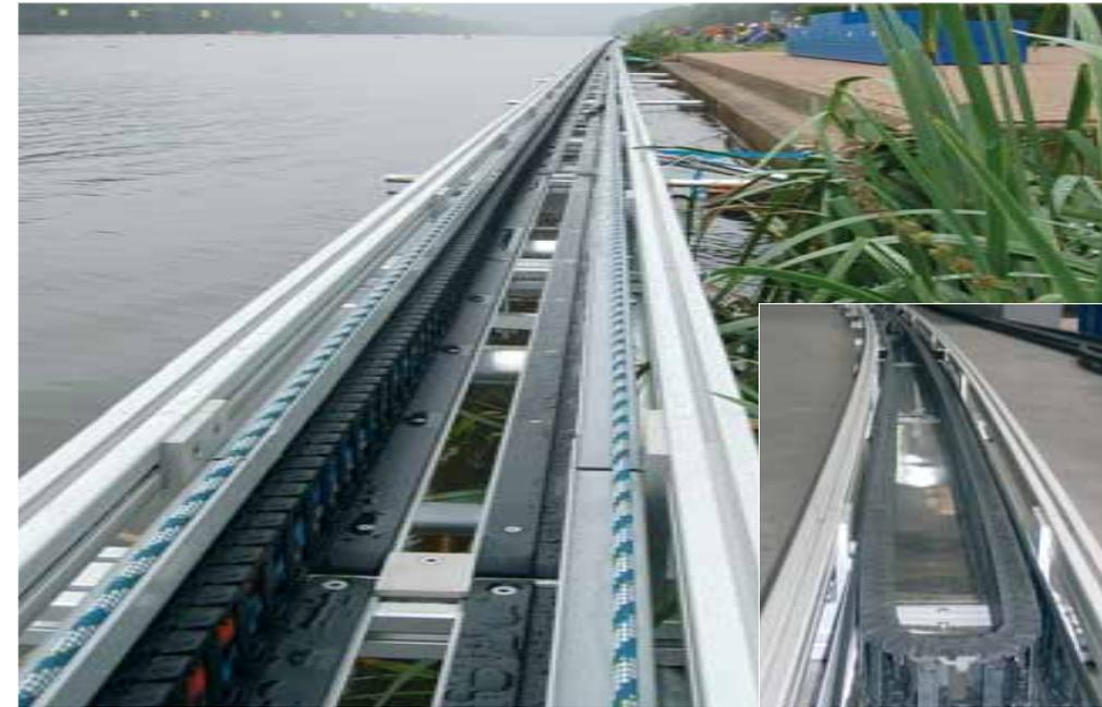
Long travel and side mounted installation with the vibration-free and low noise Series E6.29 in this camera application
