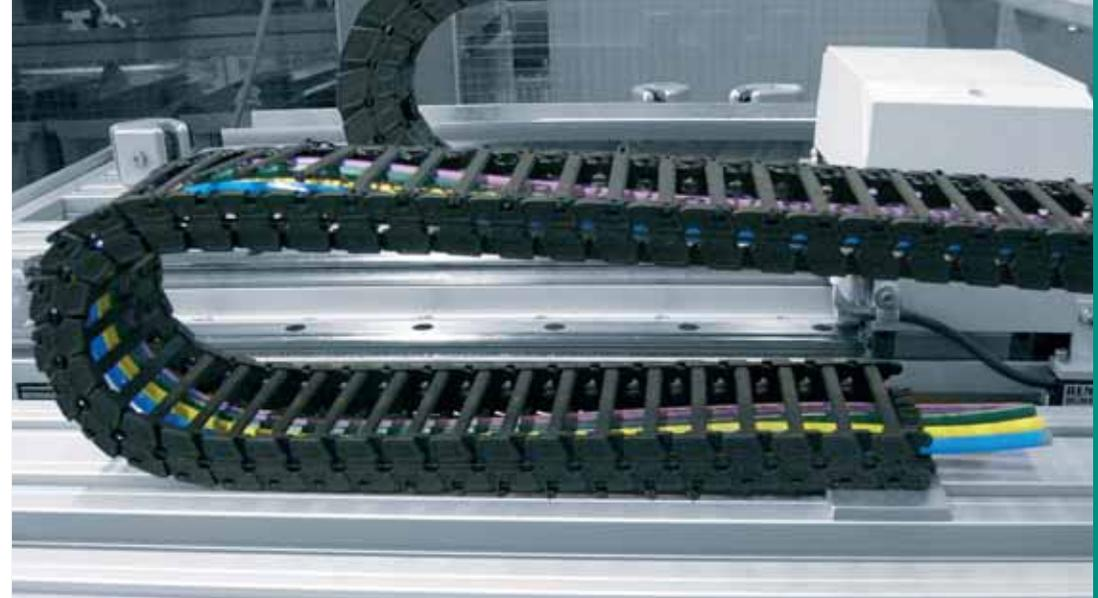
Long-term tests in our acoustics laboratory at a speed of 1.8 m/s and an acceleration of 3 m/s<sup>2</sup> showed reductions of 19-20 dB(A) compared to conventional e-chains®.
