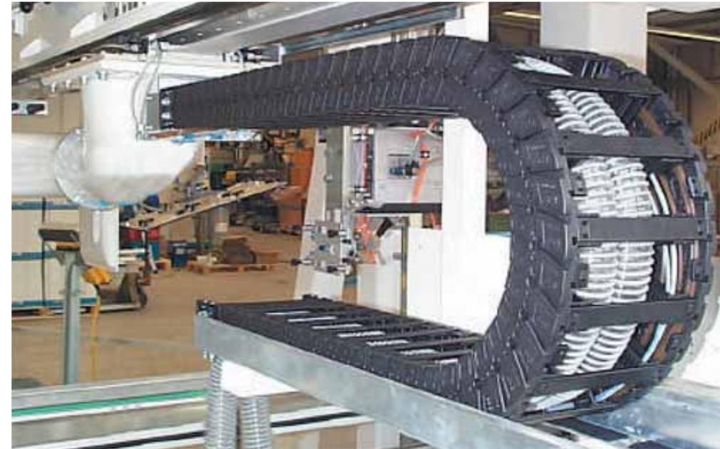
igus® System E6, pick and place robot - speed 8 m/s, acceleration 78,5 m/s<sup>2</sup>
