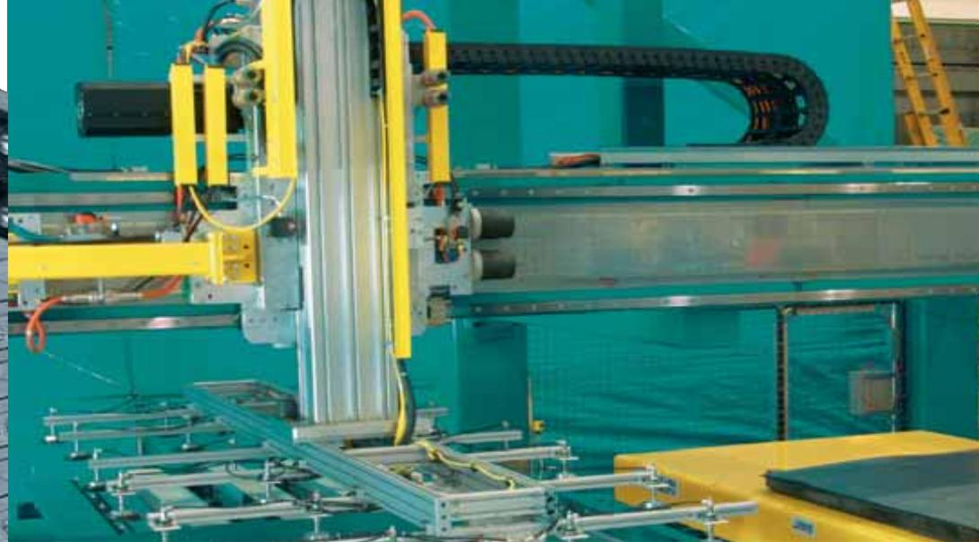
A linear drive provides for highly dynamic feed of PCBs. This system is twice as fast as handling units with a toothed-belt drive; designed to withstand high dynamic loads, the E6 e-chains® ensure a supply of power, coolant and control data with ultra-low noise and vibration
