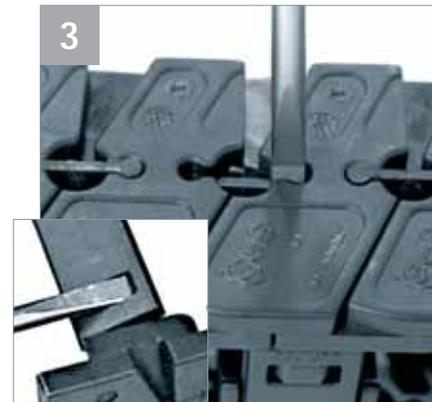
Lever crossbars with screwdriver. Tap gently to remove connectors...
