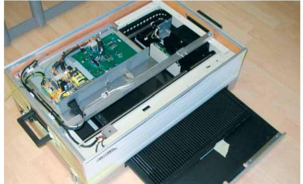
igus® Series E3.15 side-mounted in a flat-bed scanner
