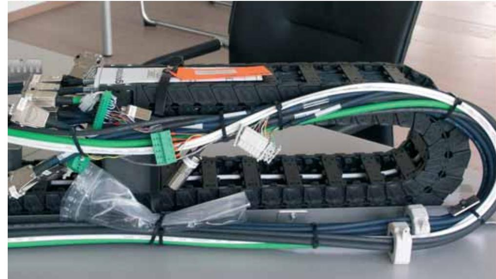
Preassembled energy supply systems reduce throughput and assembly times significantly. Because in this positioning system, cleanroom compatibility is required, each preassembled e-chainsystem is attached with a cleaning protocol.
