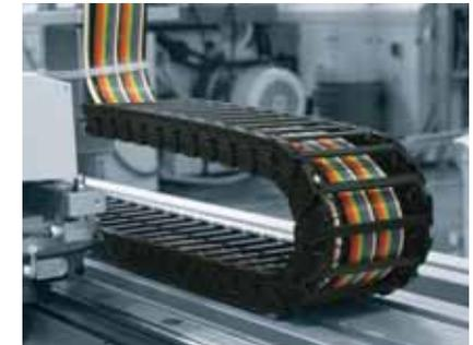
During long-term tests the System E3 with the spring band connector easily passes 15 million cycles at a bending radius of 44 mm and an acceleration of 4 g
