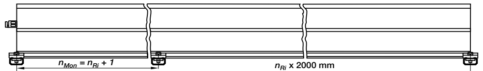
Principle sketch: Number of installation sets to be installed = Number of trough sections + 1
