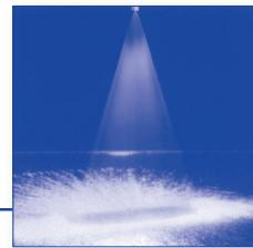
**Sharp uniform flat fan with an extremely narrow jet depth.**
