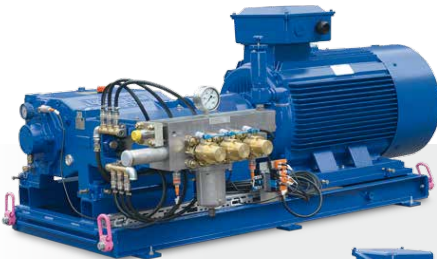
High-pressure pump unit KD724 with suction valve release for fast and accurate load changes as well as sensors for operating data logging
