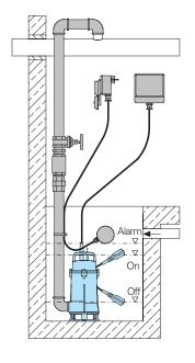
Permanent sump installation with auto-coupling system.
